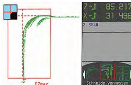
Software function for determining and measuring the tool contour
