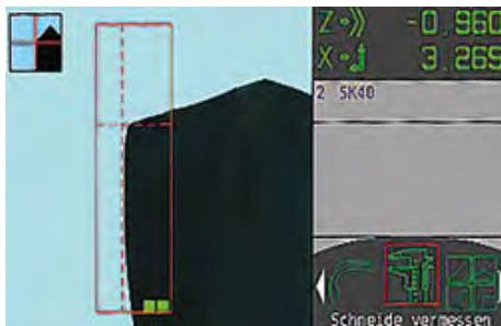
Dynamic crosshairs for automatic and fast measurement independent of the operator
